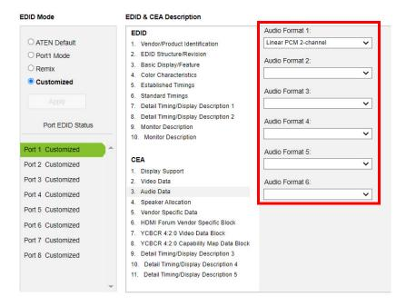
Use the drop down menu to select the **Audio Format**  $(1\sim6)$  applicable to your audio output device, and click **Save** to apply the changes.
