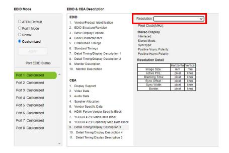
In the **Resolution** drop down menu, choose a resolution with values that fit the attached monitor/display device and click **Save**.
