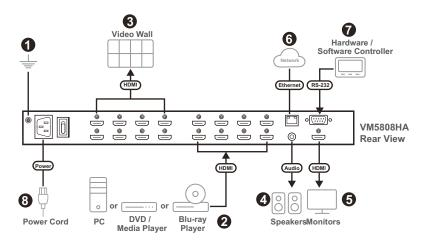
1. Use a grounding wire to ground the unit by connecting one end of the wire to the grounding terminal, and the other end of the wire to a suitable grounded object.
