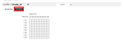
In Grid View, the audio and video outputs are assigned by mapping the audio / video input on the vertical axis to the audio / video output on a horizontal axis.
