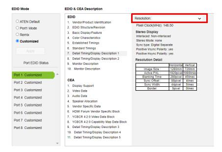
In the drop down menu, choose a resolution with values that fit the attached monitor/display device and click **Save**.
